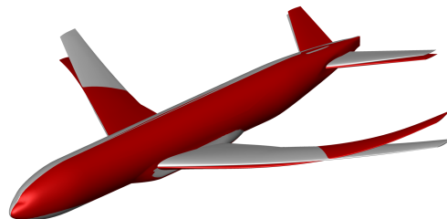
Elastic mode 2, f = 1.455 \text{ Hz} , Antisymmetric wing bending
