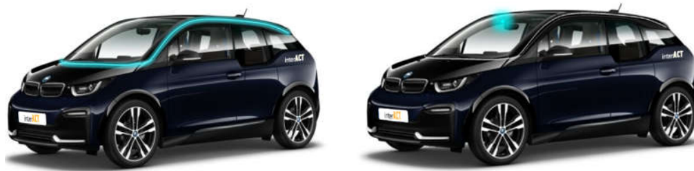
Fig. 8 eHMI variants – 360° light band (left) and directed signal lamp (right) for the interACT demonstrators
