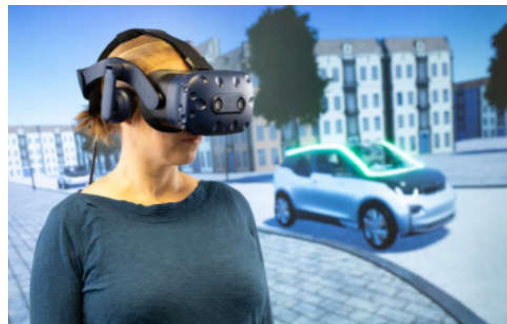
Fig. 9 Testing different eHMI variants in a VR pedestrian simulator, using a Head Mounted Display
