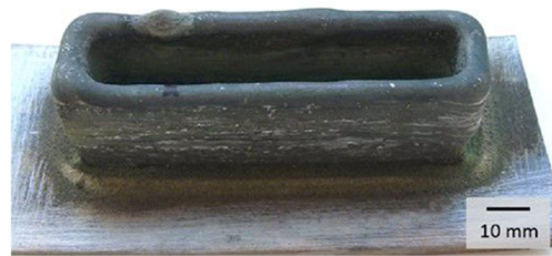
Fig. 2 Structure manufactured by 3DPMD
