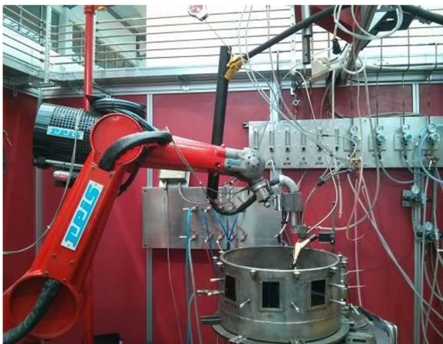
Fig. 1 Experimental setup for 3DPMD. Adapted from [2]
