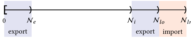
Fig. 4. Local index handling: On each MPI rank, we enumerate all locally relevant dofs with a local index [0, \mathcal{N}_{lr}) subject to the following constraints: \mathcal{N}_i is a multiple of k , the width of the SIMD registers and the interval [0, \mathcal{N}_i) only contains dofs with standard connectivity ( \#(\mathcal{I}(i)) = 3, 9, \text{ or } 27 ). A subsequent renumbering ensures that [0, \mathcal{N}_e) contains all exported degrees of freedom of the internal range. Ranges with dofs that have to be exported or imported during MPI synchronization are marked in blue and red, respectively.
