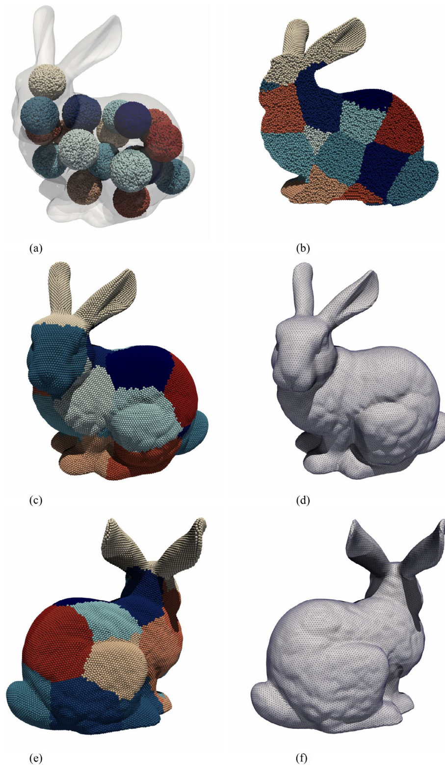
Fig. 8. bunny_20mpi : (a) Initial particle distribution. Particles are plotted with sub-domain colors. (b) Cross-section view of the particle distribution after 100,000 iteration. Front view of resulting mesh after 100,000 iteration plotted with (c) particles and (d) surfaces with edges. Back view of resulting mesh after 100,000 iteration plotted with (e) particles and (f) surfaces with edges. (For interpretation of the references to color in this figure legend, the reader is referred to the web version of this article.)
