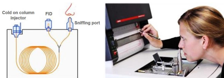
Figure 5: HRGC-O, basic principle (left) and application (right) (illustration: Martin Steinhaus)
