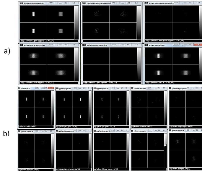
Figure 3.4: Contribution of various events with collimator and phantom medium: a) low photopeak energy (113 keV) and b) high photopeak energy (208 keV).
