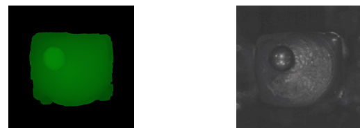
(a) Exemplary 3D-scan of a hairpin with a WS (b) Exemplary black and white picture of a hairpin with a WS
