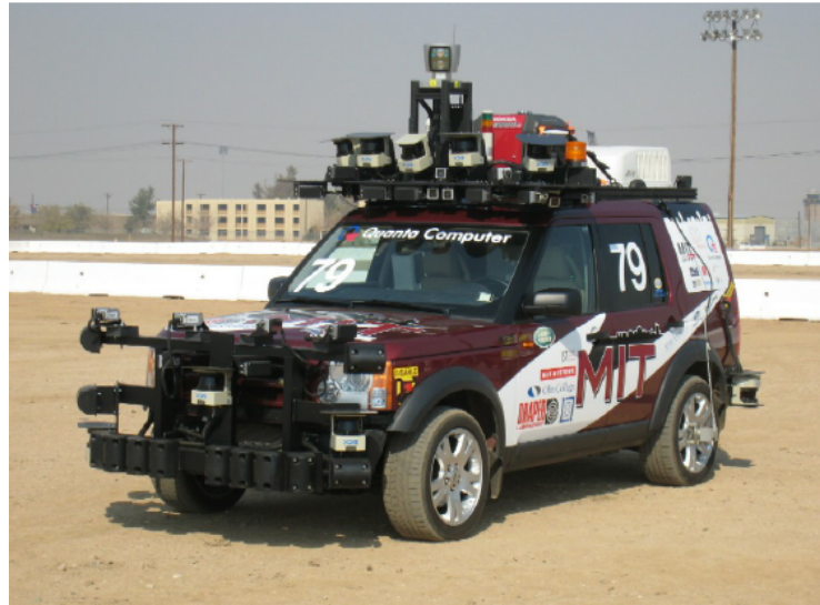
Figure 2.1: Talos, the experimental vehicle which participated for the Massachusetts Institute of Technology in the DARPA Urban Challenge [14]. Its sensor equipment is far beyond the series sensor set of the basic vehicle Land Rover LR3 [15].
