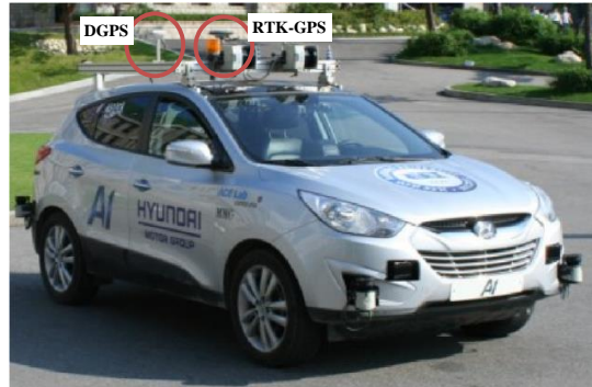
Figure 2.3: The experimental vehicle of Jo et al [9]. To enable precise GPS localization, the researchers mount several additional sensors on the vehicle. Amongst the GPS sensors marked with red circles, the figure also reveals additional Radio Detecting And Ranging (RADAR) and Light Detecting And Ranging (LIDAR) sensors installed at the front and rear bumper.
