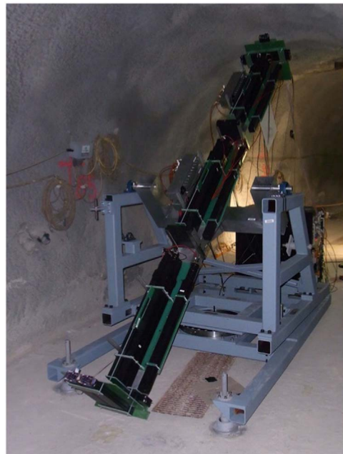
Figure 63. The 1/100 scale ‘demonstrator’ of milliQan installed in the PX56 drainage gallery 33 m from the CMS IP.
