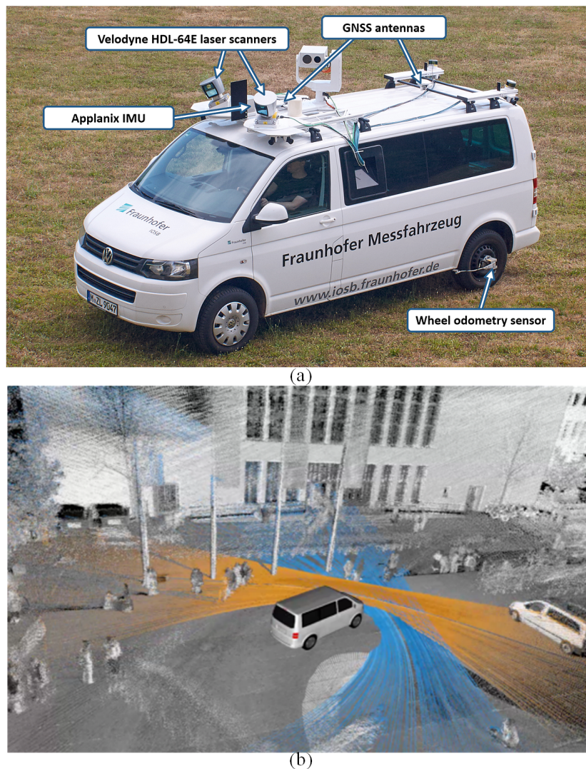
Figure 2. MLS system and its components. (a) MODISSA platform from Fraunhofer IOSB [20]. (b) Illustration of data acquisition with the two obliquely mounted laser scanners [4].
