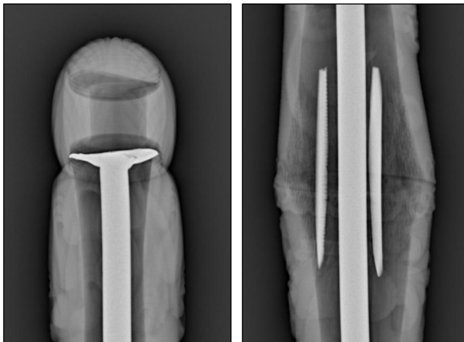
Fig. 79 (left): X-radiograph of A.1905.1144.4, bottom knob showing metal plate in detail, with inserted bone piece.
