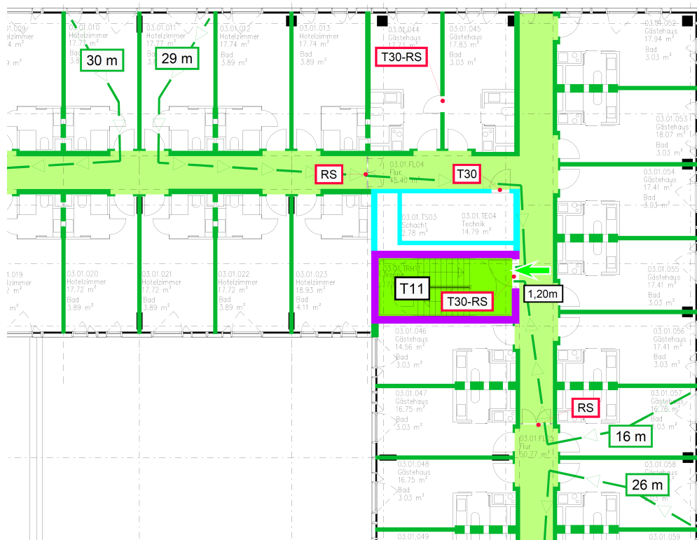
Figure 4.11: Basic concept of a fire protection plan for a hotel with a necessary hall and a stairwell with the required wall fire resistance class.
