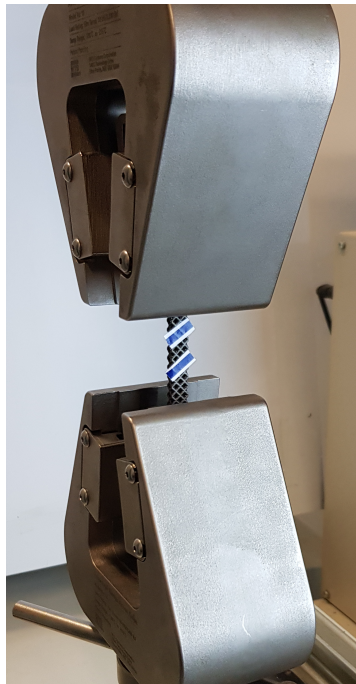
Figure 3.1: Example of a tensile experiment on manufactured AM lattice structure [86].
