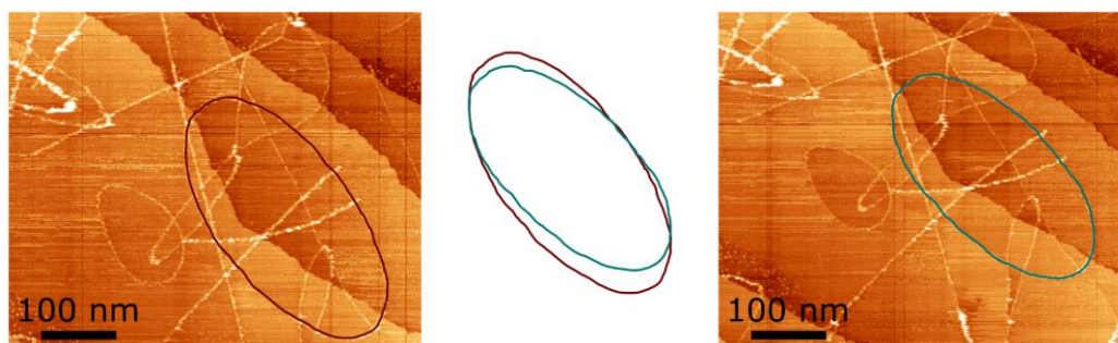
Figure 10.3 Visualization of the distortion of the STM scanner.
