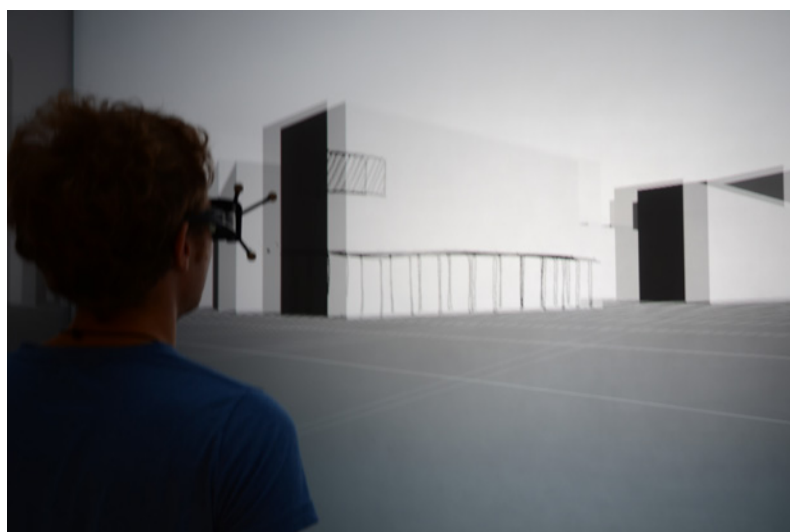
Fig. 42: Immersive view of the design scene in the CAVE. Physical models, digital ground plan and hand sketches are transmitted in real time and displayed stereoscopically.
