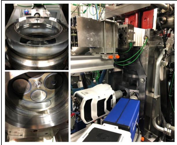
Figure 1. The optical engine. Small picture up left is the glass piston bowl, in the lower left picture the cylinder head with the injector from below; in the middle the lateral window can be seen. The picture on the right shows the arrangement of the two cameras one with the image intensifier (blue).
