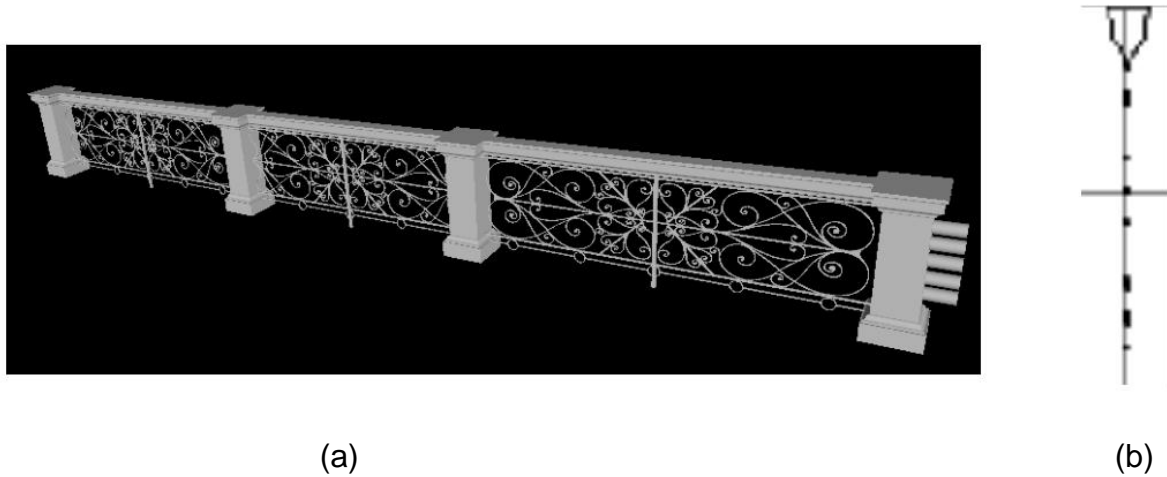
Figure 5.4: Balcony Railing building element at LOG 400 (a) 3D view (b) Slice section in the YZ plane
