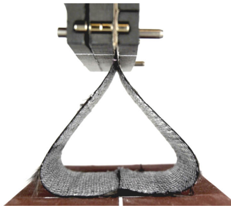
Fig. 3-12: Final configuration of a bending experiment with a \pm 45^\circ NCF sample.
