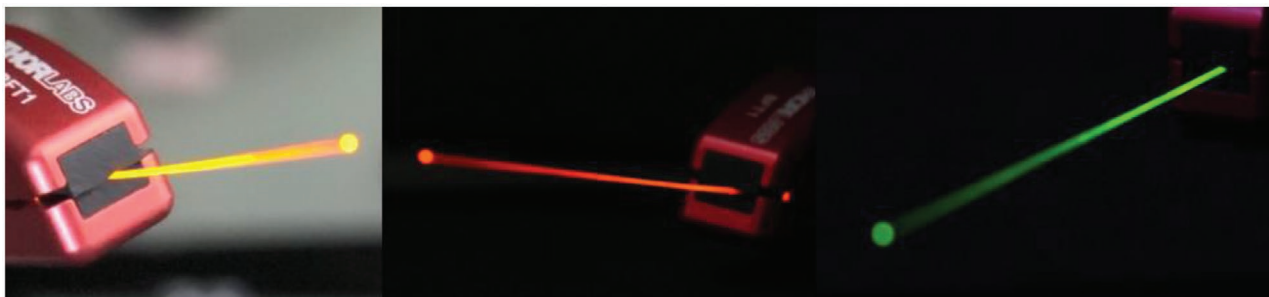
Figure 16. Light guidance through pure regenerated cellulose optical fiber.
