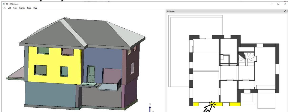
Figure 13. A prototype demonstrating the benefit of links between 2D and 3D elements for an interactive evaluation and querying purposes
