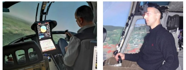
Figure 5. PAV pilots using PFD (left image) and HMD (right image) during MTEs
