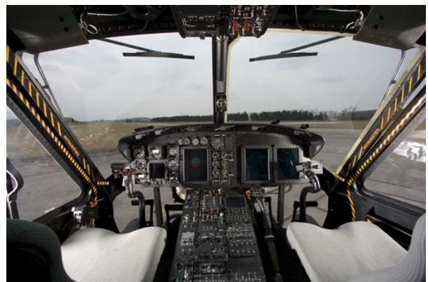
Figure 6 MAT cockpit with safety pilot environment (left side) and experimental pilot environment (right sight)
