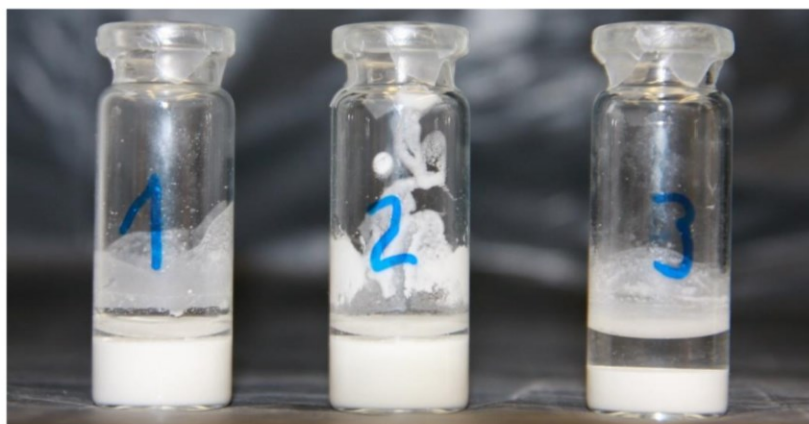
Figure 8. Hydration of fresh C_3S_m (w/b ratio = 1.0) without retarder (left), with 0.40 % bwob pyrophosphate (center) and with 0.10 % bwob gluconate (right)
