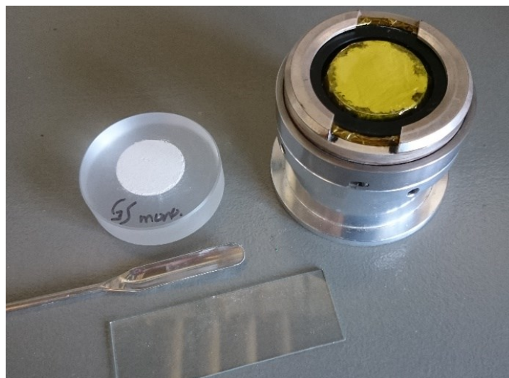
Figure 35: Preparation of powder XRD (left) and in situ XRD (right) samples.
