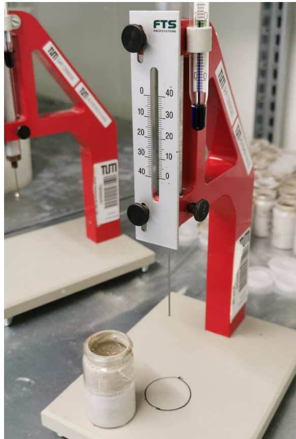
Figure 37: Vicat apparatus with glass vessel holding the hydrating sample.
