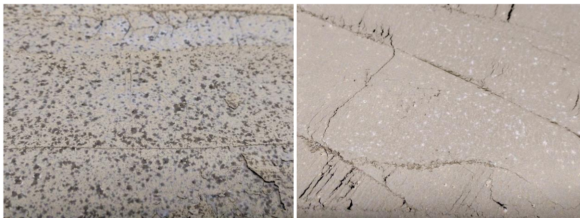
Fig. 8: Surface discolourations of the model SLU formulation (left) and of pure PC (right), appearing when aged with citrate at 35 °C and 90 % RH.
