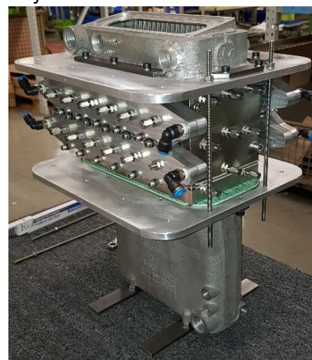
Figure 2: Condensing boiler with TEG
