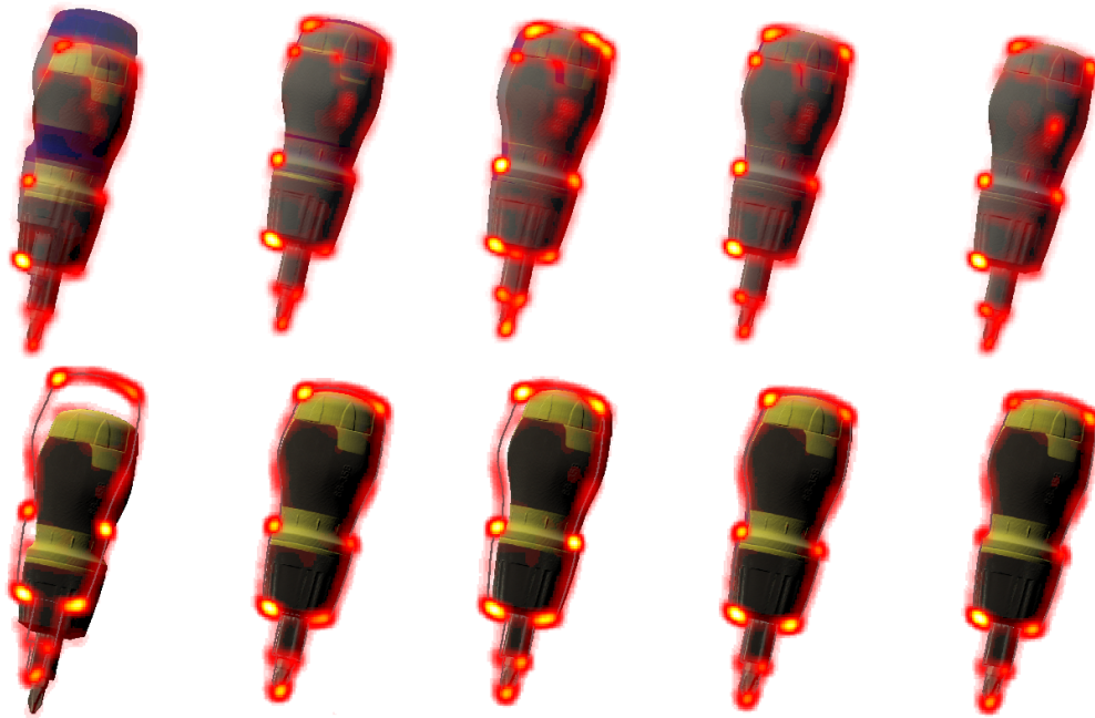
Fig. 4.8. Exemplary alignment of a screwdriver when translation errors are observed. The photometric complementary textures provide variable visual salience values that increase during the alignment process even when small misalignment errors are observed (top). In contrast, classical techniques such as silhouette visualizations provide relatively constant salience values during the alignment (bottom).
