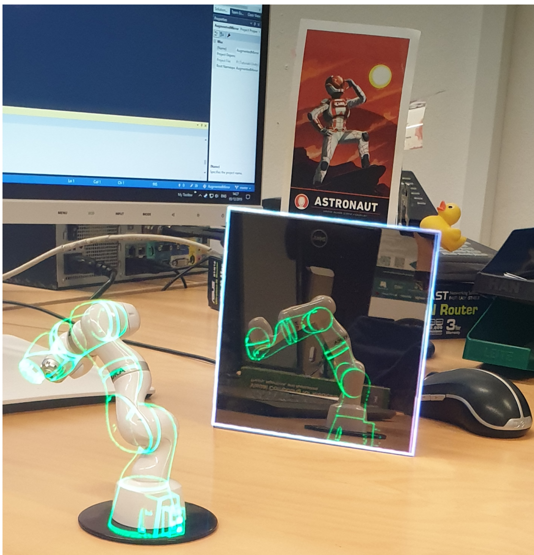
Fig. 7.3. Early implementation of an Augmented Mirror using Vuforia optical markers and an OST HMD.
