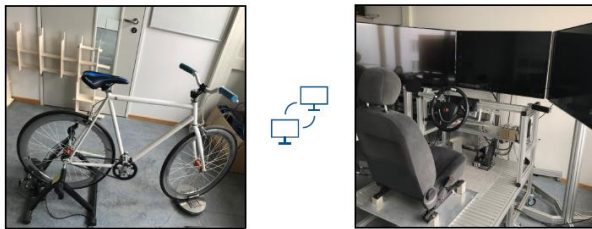
Figure 2. The bicycle simulator (left) and the driving simulator (right) used for the interconnected simulator study at the static bottleneck scenario
