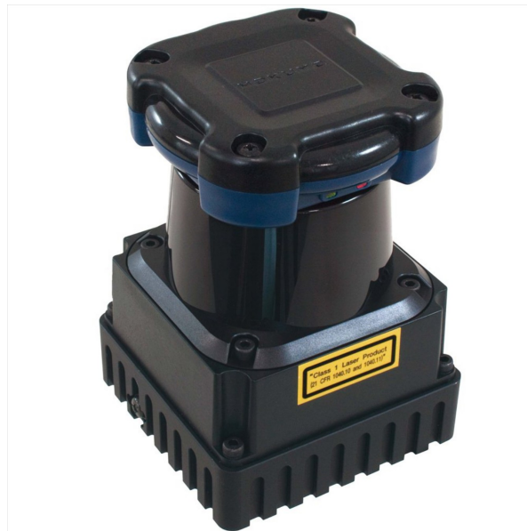
Figure 6.3.: Lidar sensor: UTM-30LX-EW from Hokuyo
