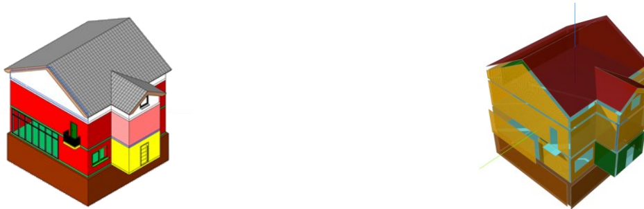
Figure 7: Preprocessing of building elements using imported parameters and view filters (l.) and visual validation using gbXML (r.)
