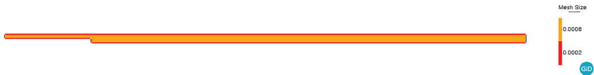
FIGURE B1 Mesh configuration for backward facing step flow [Colour figure can be viewed at wileyonlinelibrary.com ]
