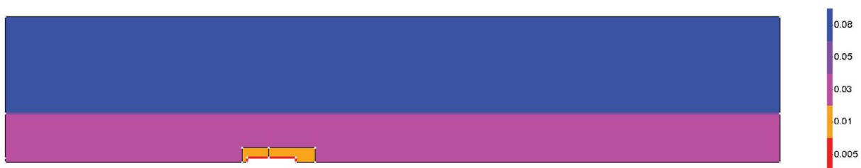
FIGURE C2 Mesh configuration for forward-backward facing step flow [Colour figure can be viewed at wileyonlinelibrary.com ]
