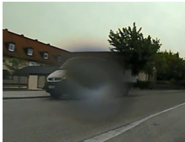
Fig. 1: Van occluded by a water droplet on the lens
