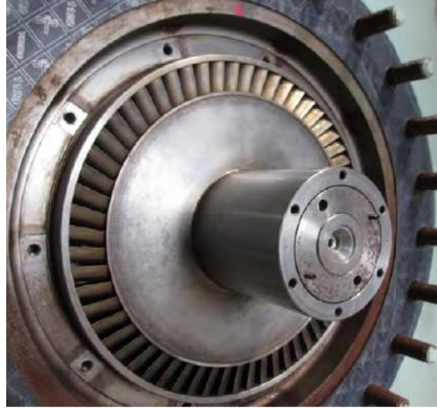
Figure 7 VPT Rotor after 4000 hour Sea Trial Operation
