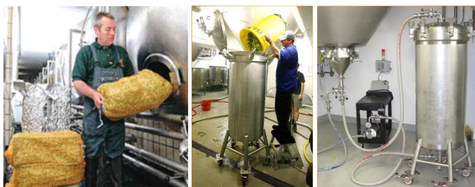
Figure 8 (1) Static dry hopping at Orval Brewery; (2, 3) dynamic dry hopping equipment at Sierra Nevada Brewery [1]
