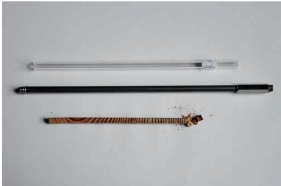
Drill core sample from the “Unterer Yngamhof” used for dating the age of the timber (from top to bottom: transport tube, drill bit, core sample).
