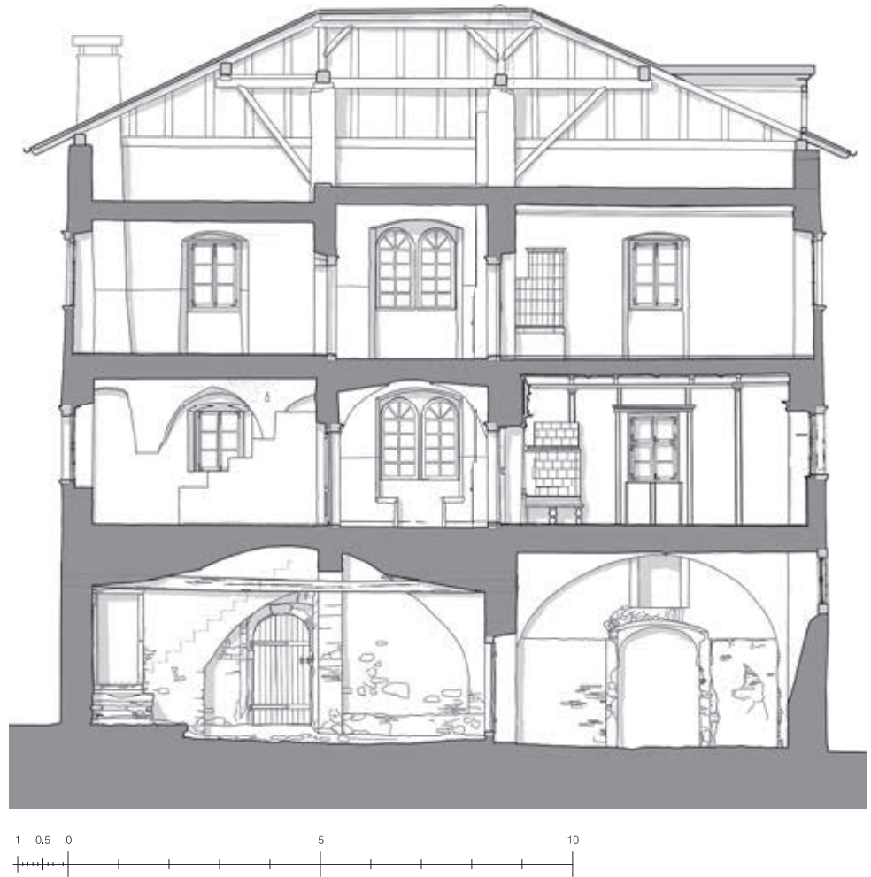
Longitudinal section of the "Unterer Yngrahamhof". The vaulted rooms of the ground floor and the hall in the middle of the house of the second and third floors are clearly visible.
