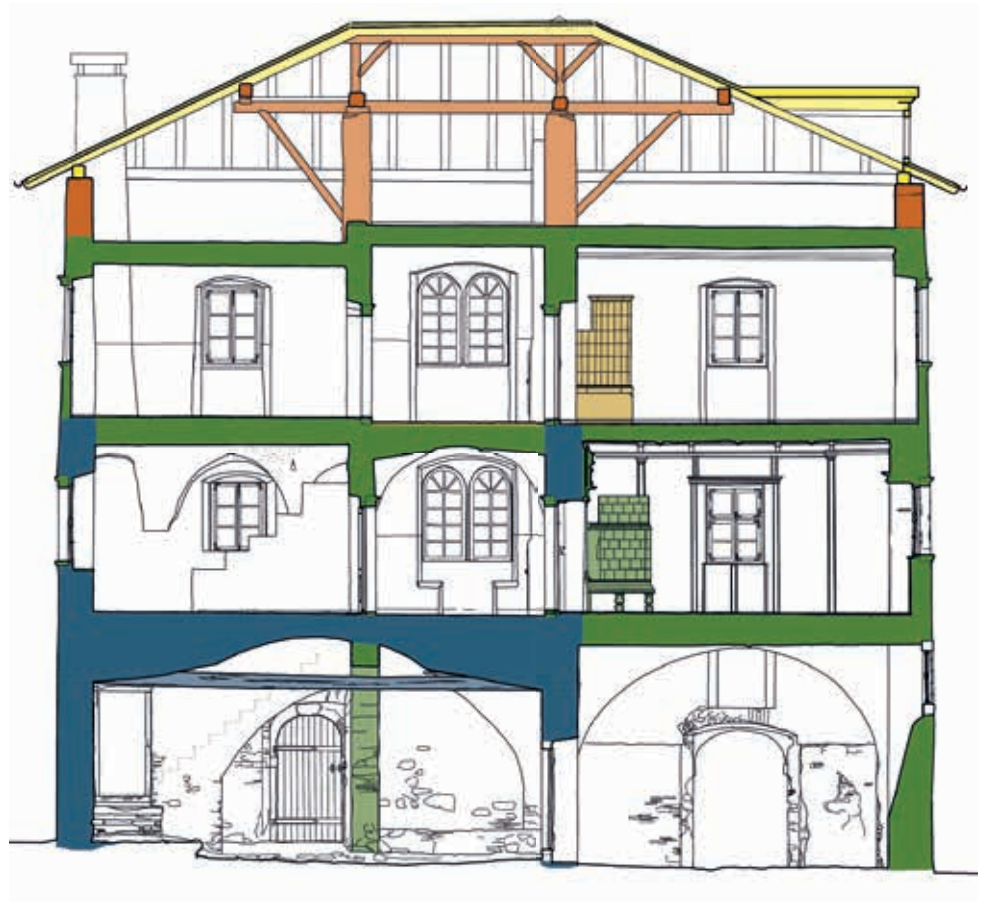
Vertical section of the "Unterer Yngramhof" in Mazon (South Tyrol), including indication of the construction phases. The original core of the building (blue) is clearly recognizable from the colored marking.
