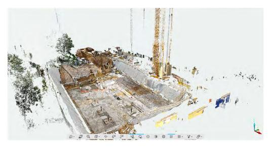
Figure 5.7: Point cloud of laser-scanner after referencing
