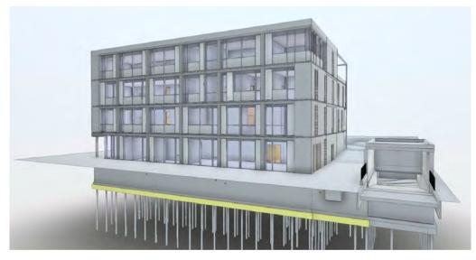
Figure 5.4: The BIM model of Building Lab Regensburg
