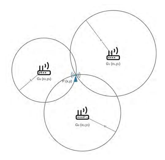
Figure 4.2: Triangulation method
