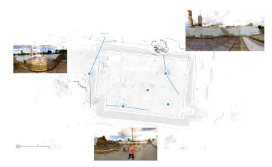
Figure 5.6: Five-point scan with Faro X130
