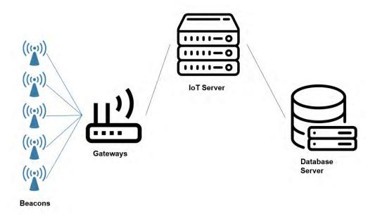
Figure 6.1: Structure of the implemented BLE system
