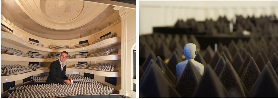
Fig. 19 Left 1:10 scale acoustic model of the Staatsoper in Berlin. The acoustician is holding a model listener whose ears are microphones for recording the sound at different places in the auditorium. Right A model listener. (Images: Peutz Associates)
