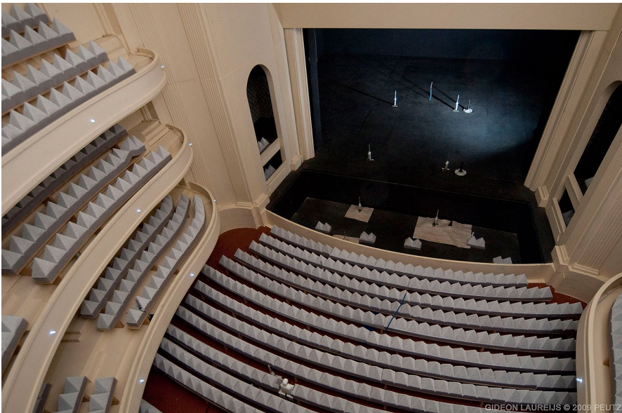
Fig. 18 1:10 Scale acoustic model of the Staatsoper in Berlin. (Image: Peutz Associates)
