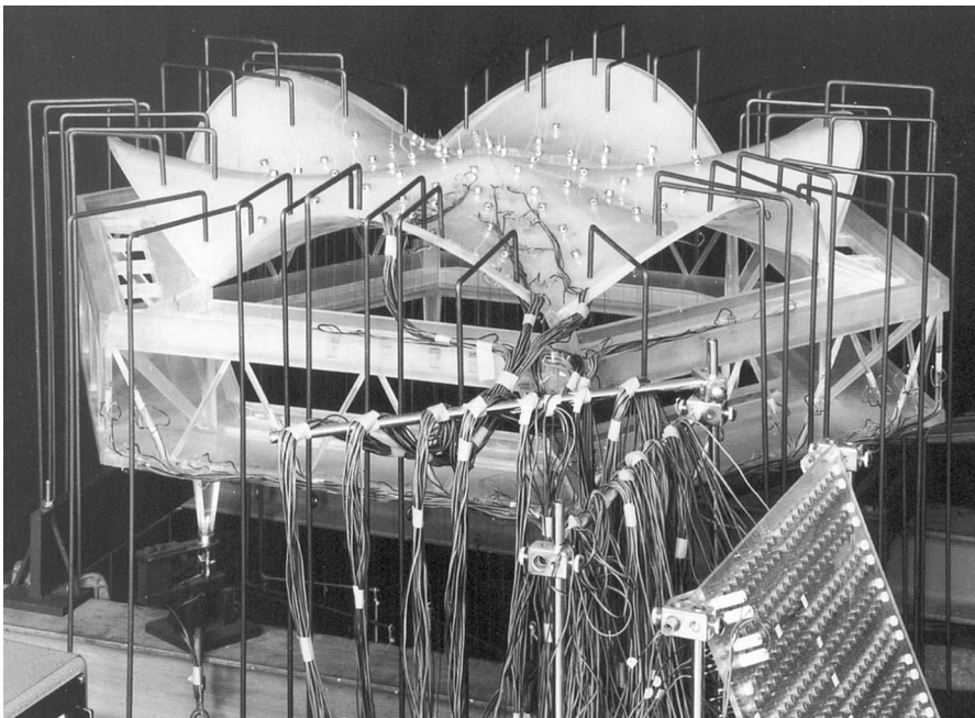
Fig. 6 1:20 Scale model in acrylic resin of the roof for the University Library, Basel, 1964. (Image: Heinz Hossdorf)
