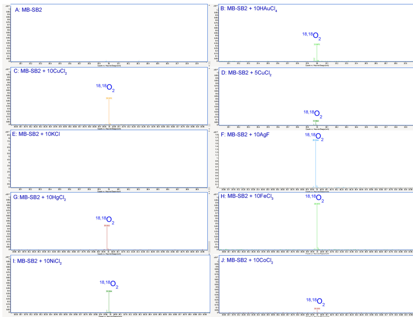
FIG 4 Mass spectra of the headspace gas of a reaction mixture containing 2 mM MB-SB2 in 97% \text{H}_2^{18}\text{O} (A) and following the addition of 20 mM \text{HAuCl}_4 (B), 20 mM \text{CuCl}_2 (C), 10 mM \text{CuCl}_2 (D), 20 mM KCl (E), 20 mM AgF (F), 20 mM \text{FeCl}_3 (G), 20 mM \text{HgCl}_2 (H), 20 mM \text{NiCl}_2 (I), and 20 mM \text{CoCl}_2 (J).
