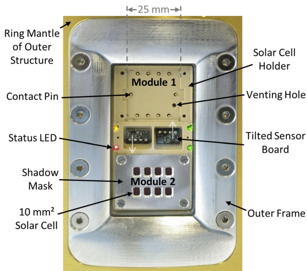
FIG. 2. Outside close-up view onto one of the eight hatches with the plugged-in insertion module. Behind the fused silica window (barely visible), the beige solar cell holder for two solar cell modules can be seen. At module position 1, the spring pins for solar cell contacts are visible, and in position 2, the shadow mask is assembled, defining eight solar cells with each 10 \text{ mm}^2 aperture. Between the solar cell modules, two tilted sensor boards (one facing upward and the other facing downward, indicated with the white arrows) are placed to collect illumination and temperature information.
