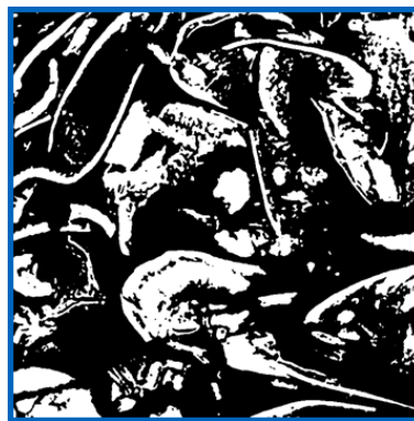
Figure 5: Binarized image of a cross-sectional slice in the interior of a spent grain filter cake. The image was generated using computed X-ray microtomography and shows the cake solids in white and air in black
