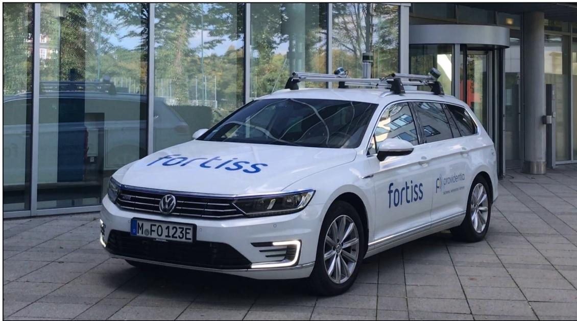
Figure 6.1: The Fortuna autonomous driving vehicle experimental platform: a modified VW Passat with lidar sensors and antennas on the roof rack, additional cameras inside the vehicle and additional radar sensors integrated in the bumpers. (graphic from [KK19], ©2019 IEEE)
