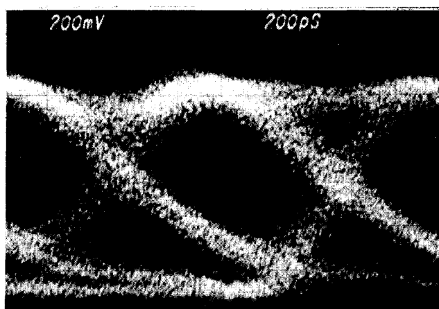
Fig. 13 Eye pattern at the input (a) and output (b) of the decision circuit
