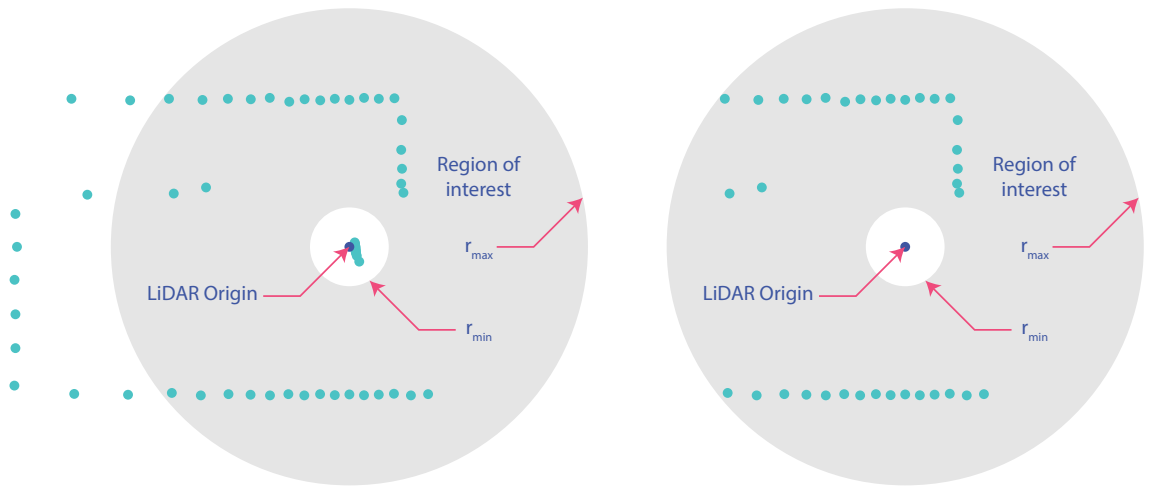
Figure 4.3: Points inside region of interest, that is, between r_{min} and r_{max} are retained. Left: Raw scan for LiDAR sensor; Right: Scan after filtering points outside region of interest
