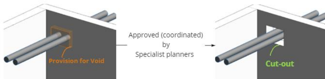
Figure 1.6: MEP Provision for void (PfV) objects (left) and cut-out as opening in the wall (right) (adapted based on the 'Guide to BIM Modeling in Revit (2020)' 2 )
