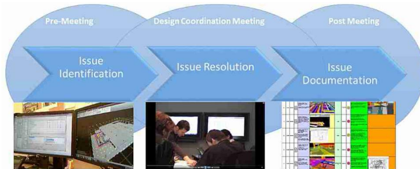
Figure 2.4: BIM-based design coordination process critical steps: issue identification, issue resolution, and issue documentation (Mehrbod et al., 2019)
