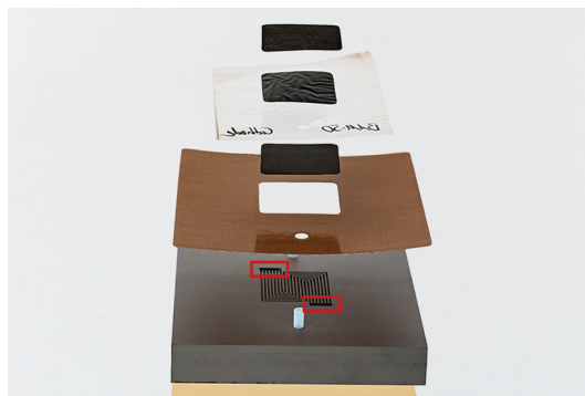
Figure 2.11. Picture detail of fig. 1.1 showing the cathode FF and the 5-layer MEA. The deep gas distribution headers at the gas inlet and outlet of the FF are highlighted in red.
