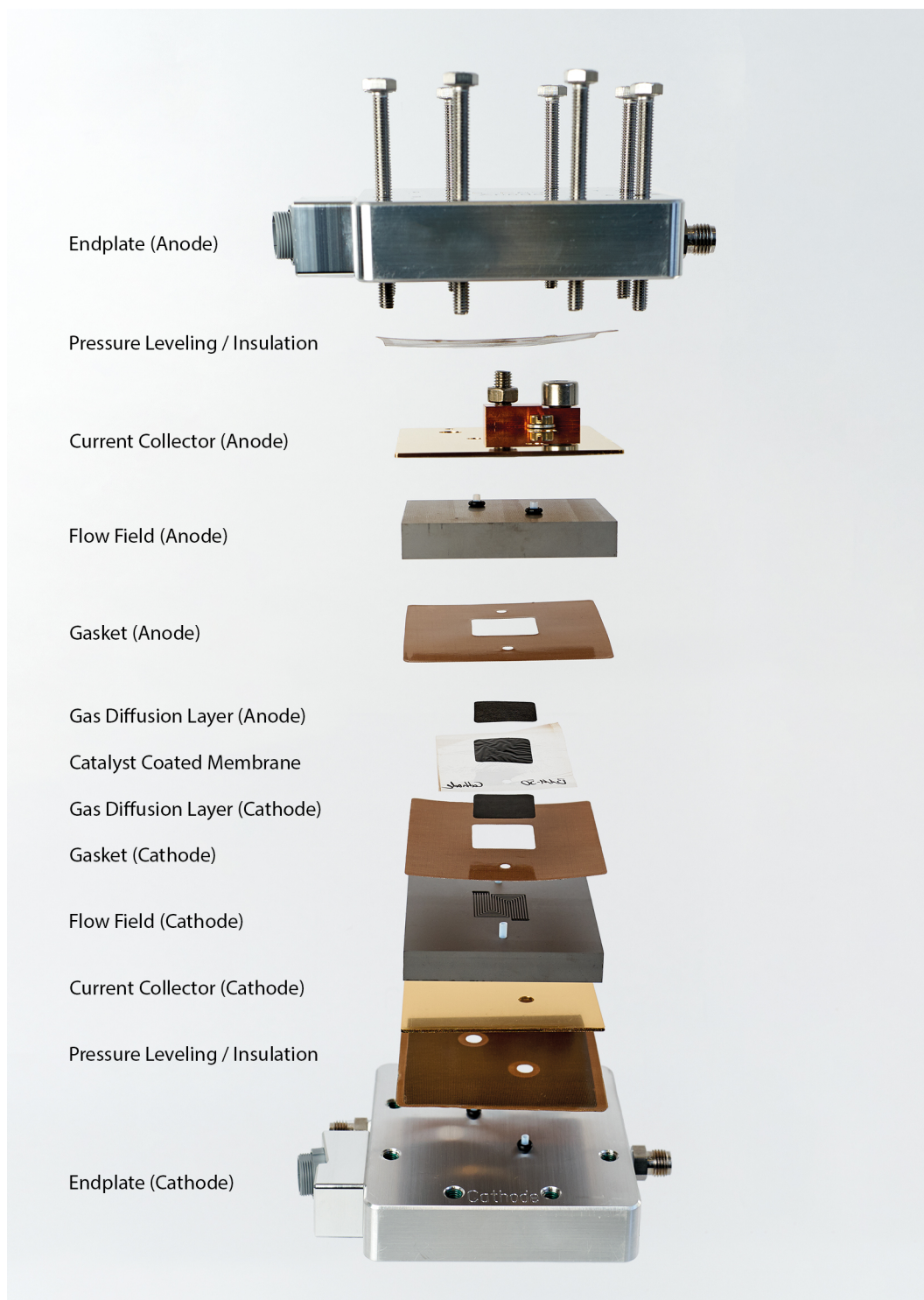
Figure 1.1. Components and assembly of the 5 cm 2 active area PEMFC hardware that was used throughout this thesis for the characterization of PEMFC single-cells.
