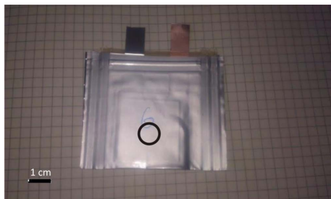
Figure 1. (color online): Assembled pouch bag cell for in situ SANS. The circle shows the neutron beam size and position on the cell.
