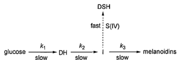
Fig. 2 A kinetic model for the glucos/glycine browning reaction, showing the point at which the reaction is inhibited by sulfite species, S (IV). DH is 3-deoxyhexosulose, DSH is 3, 4-dideoxy-4-sulphohexosulose, and I is an unspecified intermediate [72, 74]
