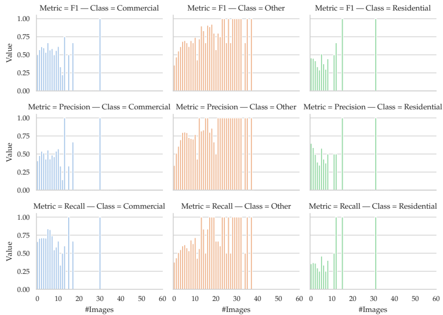
Figure 6.17: F1 score, precision, and recall as a function of the number of images per building at a class-wise level for InceptionResNetv2 model.
