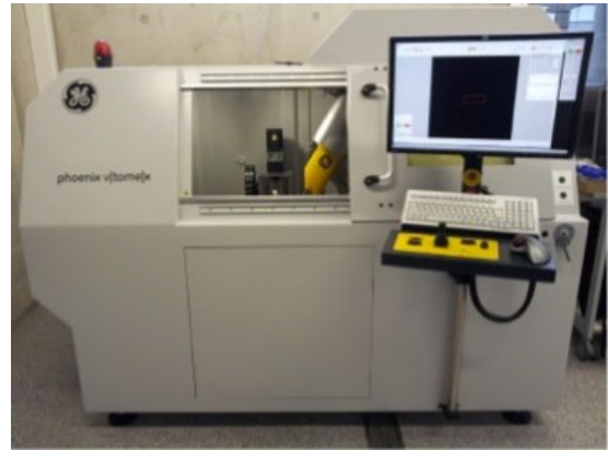
(b) Phoenix/GE v|tome|x s240 micro-CT scanner at the Munich School of BioEngineering 2
