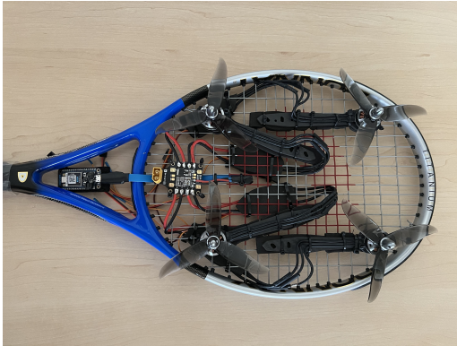
Figure 9: Testbed for force feedback system: four brushless electric motors and their respective ESCs with anti vibration foam
