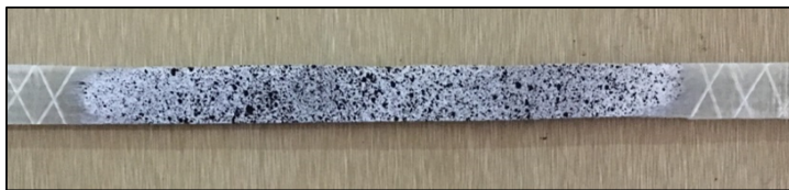
Figure 2. Tensile Test specimen — 0^\circ fibre orientation
